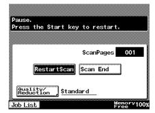
7 After scanning of the original to be transmitted is finished, touch [Scan End], then press the [Start] key.
