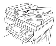
Input the fax number using the 10-Key Pad, and then press the [Start] key.
